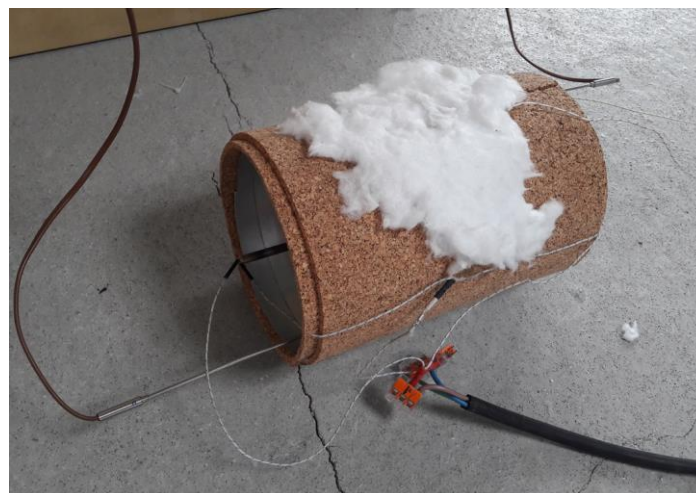
Figure 12: Illustration of the experiment (the temperature measurement on the outside of the insulation is protected of the ambient temperature with some rockwool)
